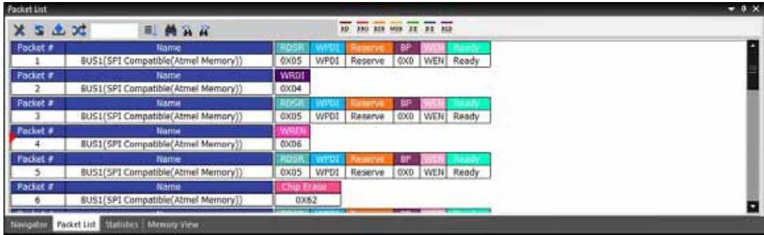
Figure 4-77 Packet List window example showing an SPI protocol
