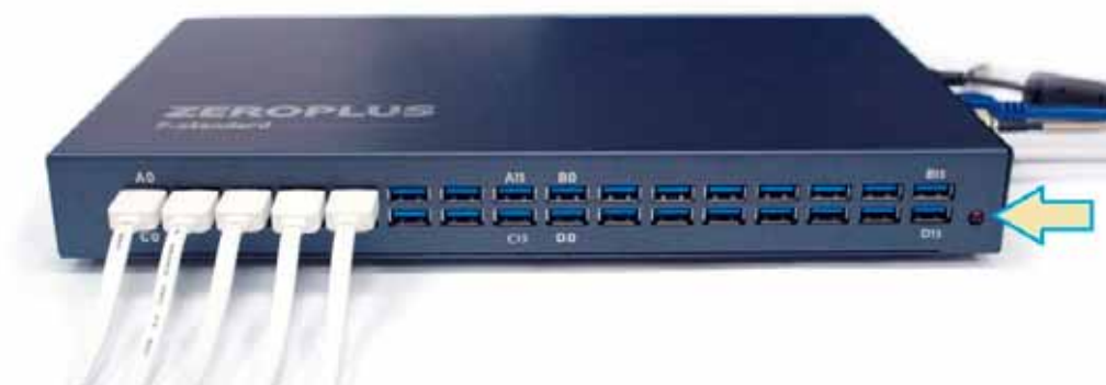
Figure 2-5 Signal cable connection and power lamp location
