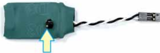
Figure 2-7 eMMC probe tuning screw
